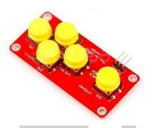
value is used. For the digital keypad you need to check each pin/key separately. For example. If left key is pressed, if right key is pressed. The analogue keypad uses a single variable which has a different value depending on the key pressed. For example. if Keypress is left, or if keypress is up. I found this a little easier to work with but it can be written anyway you wish.
